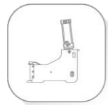
a. 双指夹料 Two-finger clamp
