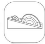
d. 小锯独立运动 scoring saw independent moving
