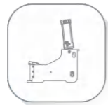
a. 双指夹料 Two-finger clamp
