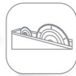
b. 小锯独立运动 scoring saw independent moving
